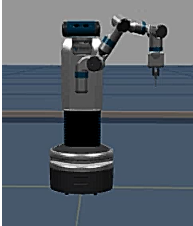
Figure 7: Experimental setup for the screwdriver task. The robot is initialized to this pose, which is similar to the initial pose of other experiments done in the Laboratory for Progress. The robot starts with the screwdriver grasped by the gripper.
