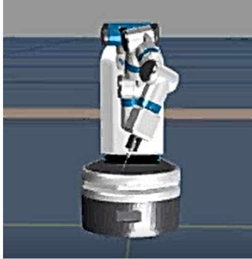
Figure 8: End state of the screwdriver task. The goal position has been reached by the motion potential while performing the screw action. The axis potential did move the end-effector along the screwdriver’s axis of motion, but notice that the screwdriver is not aligned with the vertical axis.
